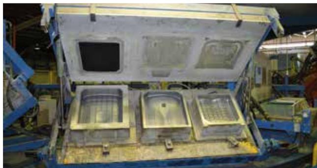
Moulded foams, although more expensive to create and manufacture, can be made with much greater precision. Precise shapes, such as an anatomically formed pelvic well or abductor/adductor contouring, provide better support and fit. Also, the top finish adds durability and is easier to wipe clean compared to cut foam.
